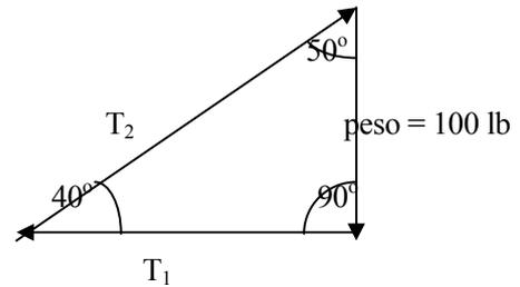
$$\frac{T_1}{\text{sen}50^\circ} = \frac{\text{peso}}{\text{sen}40^\circ} \Rightarrow T_1 = \frac{\text{peso}}{\text{sen}40^\circ} \cdot \text{sen}50^\circ = 119.17 \text{ libras}$$
