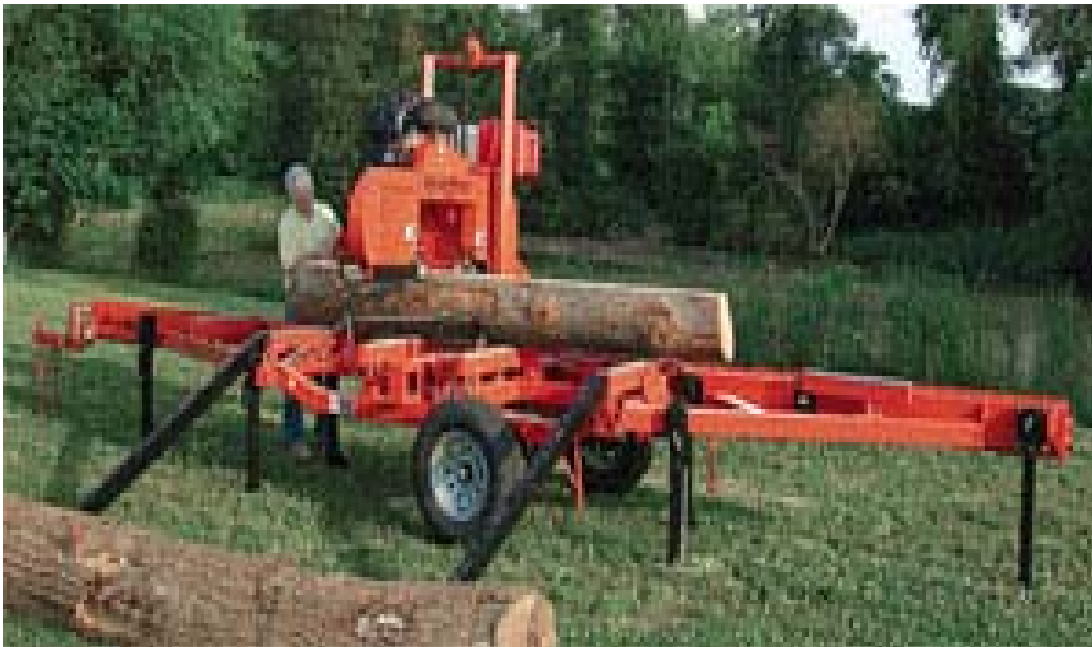
Figura 4. Aserrío portátil Wood-Mizer LT40. Fuente: Wood-Mizer Products, Inc. 2007.
